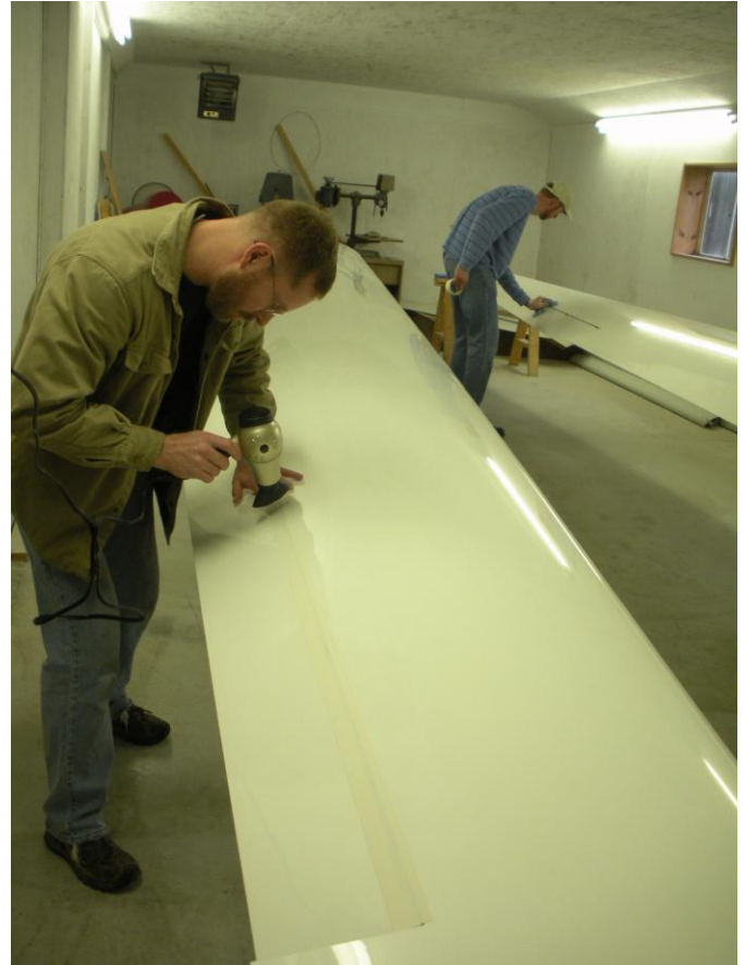
John Dudley and Chris Uhl apply new tape to aileron joints of "CC" wings
